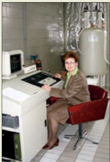
Bruker AC 250 E NMR Spectrometer (Operator: Prof. Mirjana Popsavin)
